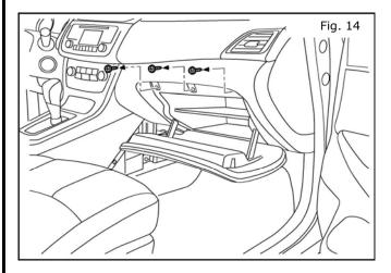
14. Open the glovebox door. Remove three (3) phillips head screws from inside the glovebox compartment.
