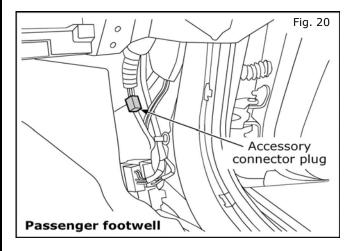
20. Locate the **passenger side** Accessory Connector plug. It will be below the glovebox on the right side.
