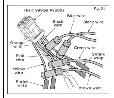
21. Using a posi-tap, connect the **Black** wire from the power harness to the **Black** wire on the Accessory Connector Harness.
