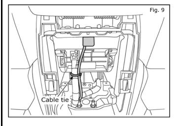
9. **Install** the encoder so that the shaft is inside the back of the armrest storage compartment.
