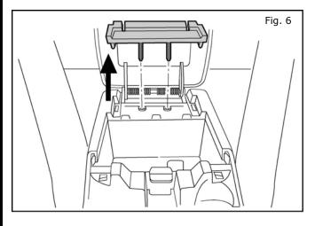
6. Remove retainer clip panel at the back.
