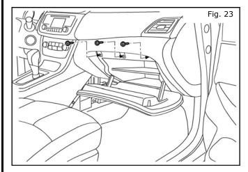
23. **Reinstall** the glovebox. **Reinstall** three (3) phillips head screws from inside the glovebox compartment.
