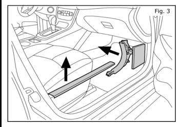
3. Carefully remove passenger side door sill trim panel, the outer footwell panel and the foam cover panel as shown.
