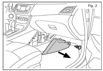
Carefully pry out retainer clip and center footwell panel from the passenger side of the center stack.
