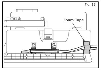
18. Secure the harness to the back of the glovebox with foam tape as shown.
