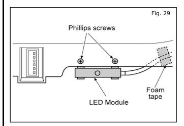
29. Place the driver side LED module on the **inside** of the panel with the LED facing **downward**. Use two (2) phillips screws from the outside of the panel to mount the driver side LED module.
