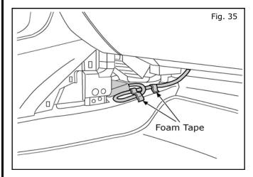
35. **Bundle** any excess wiring and secure with foam tape under the center stack as shown.
