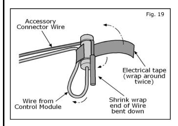
19. Follow this finishing procedure on all posi-taps. Leave a short length of wire extended past the posi-tap and bend down as shown. Use electrical tape to secure the extra wire against the posi-tap with at least two revolutions.
