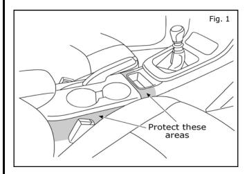
1. CAUTION: BE SURE TO PREP INTERIOR SURFACES WITH PROTECTIVE CLOTH OR LOW TACK MASKING TAPE TO PREVENT ANY SCRATCHING OR BLEMISHES TO THE INTERIOR
