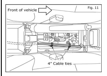
11. Route encoder wiring harness forward through the center console and up towards the center stack. Secure with two (2) 4" cable ties, as shown.
