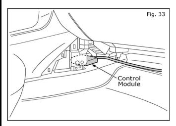
33. Peel the cover off the tape on the controller. Securely place the controller on the carpet under the center stack.
