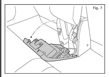
7. Carefully pry off cover panel from the rear of the center console.
