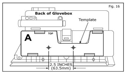
16. Trim out template "A" and tape in place on back of glovebox as shown. The template should be positioned along the bottom and left edge with the letter "A" in the upper left hand corner.
