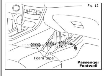
12. Route encoder wiring harness up through the center stack and out to the passenger side footwell. Secure harness inside center stack with foam tape.
