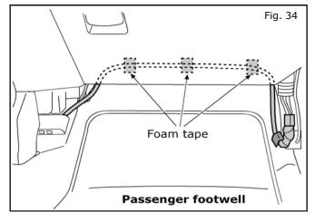
34. Route the wiring that leads to the Accessory Connector up behind the glovebox. Secure the wiring with foam tape.
